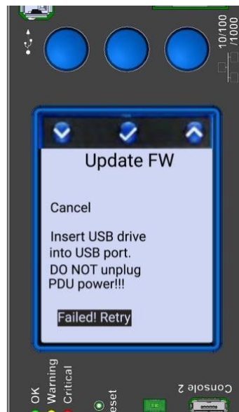
Sample of Failed updating
