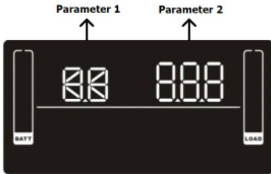
There are three parameters to set up the UPS. Parameter 1: It's for program alternatives. Refer to below table. Parameter 2 is the setting options or values for each program.
