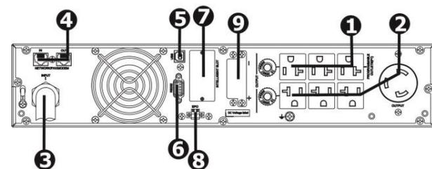
1. Programmable outlets: connect to non-critical loads
