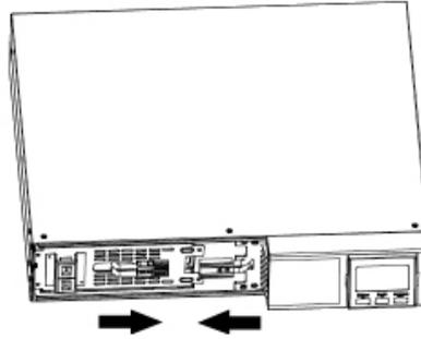
Re-connect the battery wires.
