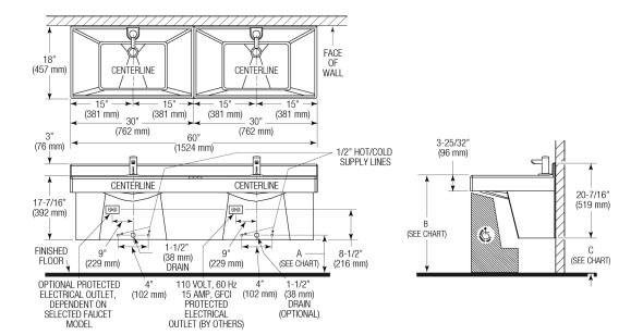
110 VOLT, 60 Hz 15 AMP, GFCI PROTECTED ELECTRICAL OUTLET (BY OTHERS) OPTIONAL PROTECTED ELECTRICAL OUTLET, DEPENDENT ON SELECTED FAUCET MODEL
