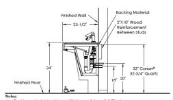
Backing material should equal thickness of drywall, 1/2" min.
