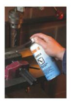
The **TUFCUT** range is comprised of specialist metal cutting lubricants based on a mixture of extreme pressure additives and anti-oxidants. They have been formulated with high film-strength and resistance to extreme pressures, that extends tool life, dissipates heat and prevents chip welding. Tufcut allows heaver, close tolerance cuts, reducing rejects and increasing production.
