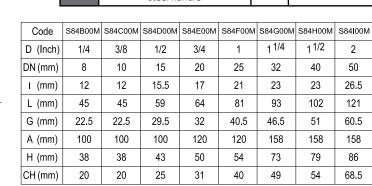
Ask for additional information on the whole range of *RuB* valves and consult with your supplier for special applications. Ball valves are marked CE on handle from 1.1/4" to 2" as follow: CE XXCODEXX Cat I-A
