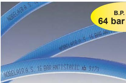
Antistatic PVC hose for arduous uses, comprising three thermoplastic layers, reinforced with a high resistant textile polyester braiding. Its inner lining is smooth and conducts electricity.
