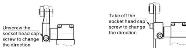
3 Installation position of leverage can be changed.
