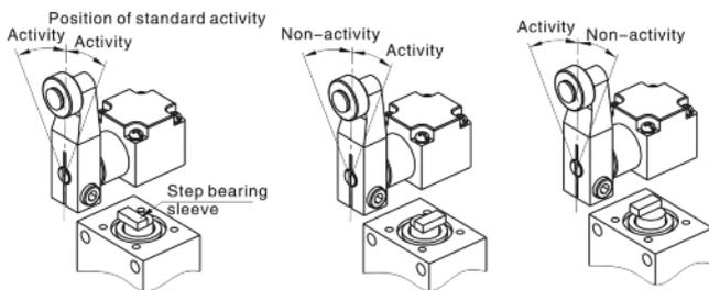
2 The rolling wheel can be installed at the inside of leverage.
