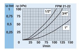
N.B. All the curves have been obtained with mineral oil having a kinematic viscosity 30 cSt and specific gravity 0,9 kg/dm³; for fluids with different features, please consider the factors described in the first part of this catalogue. All the curves are obtained from test done at the UFI HYDRAULIC DIVISION Laboratory, according to the specification ISO 3968:2005. In case of discrepancy, please check the contamination level, viscosity and features of the fluid in use.
