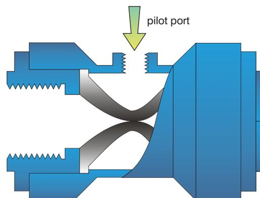
Valve with pilot signal is normally closed
