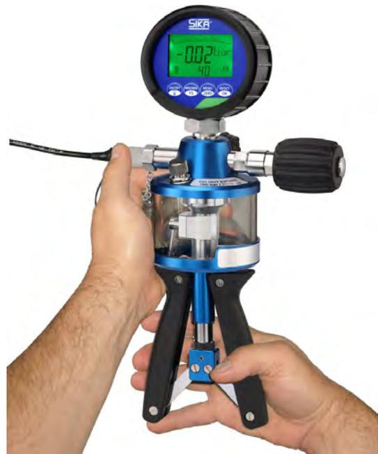
**TIP!** At high pressures, open the handle only lightly.
